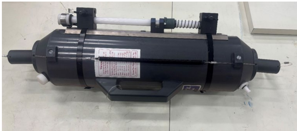
Figure 14-Niskin bottle water sampler used for water quality sample collection
