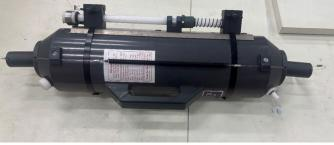
Figure 14-Niskin bottle water sampler used for water quality sample collection
